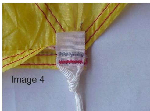
Image 4: Compliance with this Service Bulletin requires adding a 42 stitch bartack in 16 places, one at each of the eight 'A' line loops and one at each of the eight 'B' line loops.
